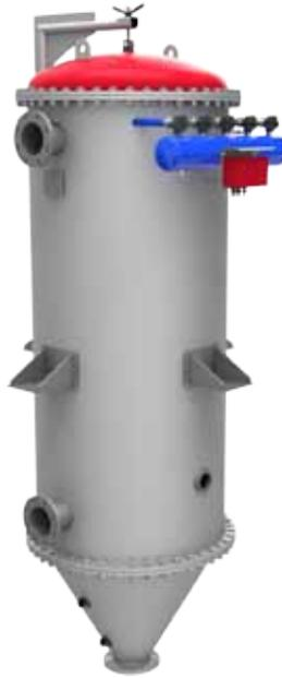
dedusting of two pneumatic pressure conveyings two silo vent filters type Infa-Mini-Jet AJM to this company. Because of the flammability of isophthalic acid, the preventive explosion protection was specified by inertisation with nitrogen. Special feature is conveying and filter cleaning with nitrogen. That's why the filters are designed gastight.
